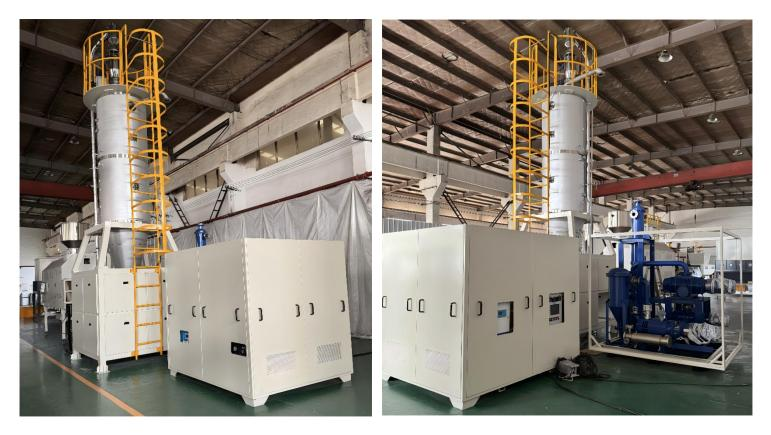
LIANDA MACHINERY integrates Infrared crystal dryer (IRD) with the SSP system, which uses infrared wave to quickly and evenly heat the material, shorten the pre-treatment time, and optimize the mass transfer efficiency in the solid phase reaction, making the entire system highly energy-efficient, with large processing capacity and high product stability. It is especially suitable for large-scale high-quality production of recycled PET.
